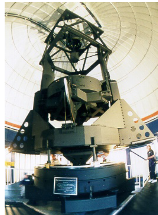
The 1.8 meter Spacewatch telescope which is used for NEOs identification and tracking.
